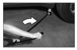
Raise the vehicle by turning the jack handle clockwise. Raise the vehicle far enough off the ground so there is enough room for the spare tire to fit. 6. Remove all the wheel nuts and take off the flat tire.
